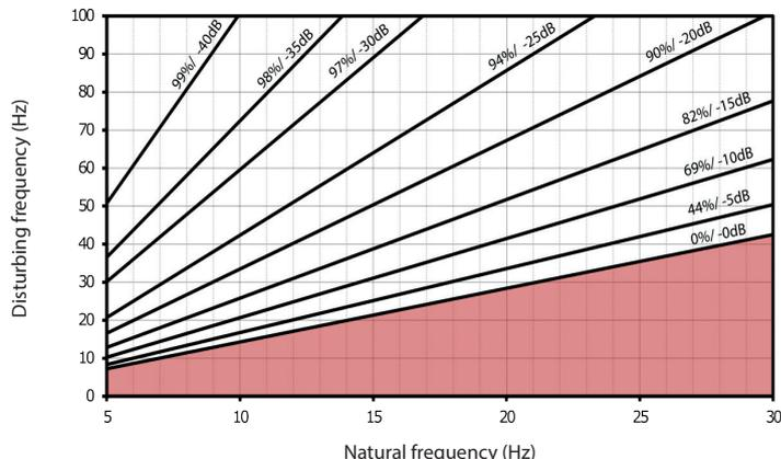
Vibration isolation efficiency by implementation of an elastic bearing made of VibraFlex® VF25 on a rigid base.
