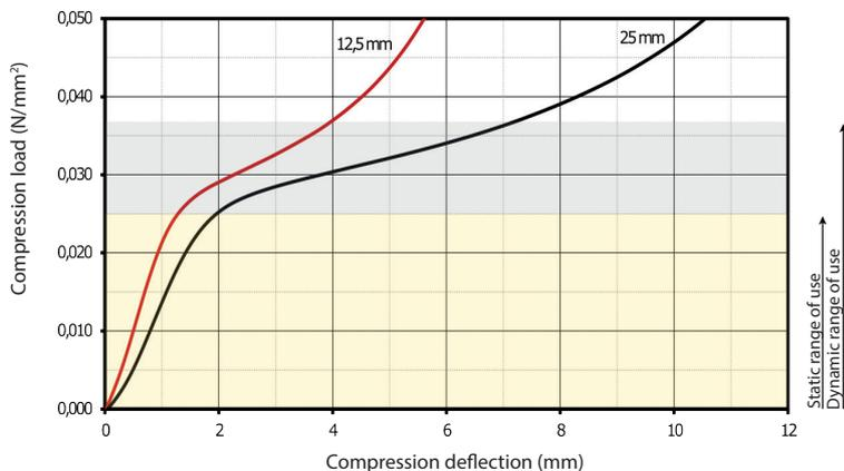
Static compression load deflection of 3<sup>rd</sup> load occurrence. Testing between flat and plane-parallel steel plates.
