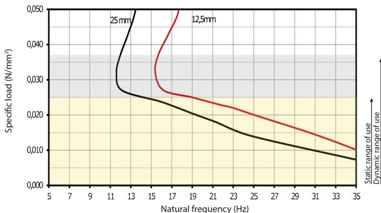
Natural frequency of a single degree-of-freedom system (SDOF System) consisting of a mass and an elastic bearing made of VibraFlex® VF25 on a rigid base.
