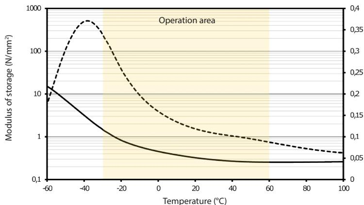
DMTA graph shows the relation between storage modulus and tan delta over temperature.
