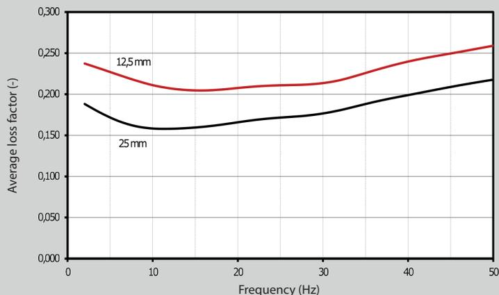
Mechanical loss factor is measure for energy loss per cycle in an oscillating system.
