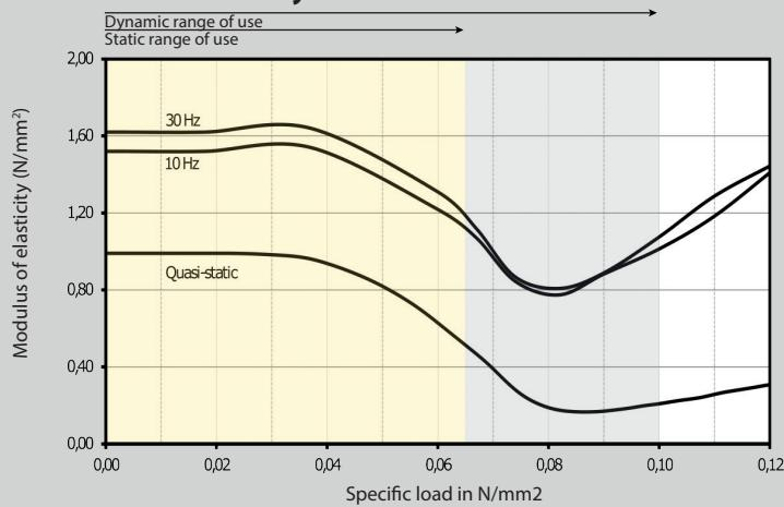
Dynamic modulus of elasticity for a sinusoidal excitation at a constant mean load and an amplitude of ± 0,25 mm.
