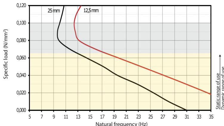
Natural frequency of a single degree-of-freedom system (SDOF System) consisting of a mass and an elastic bearing made of VibraFlex® VF65 on a rigid base.
