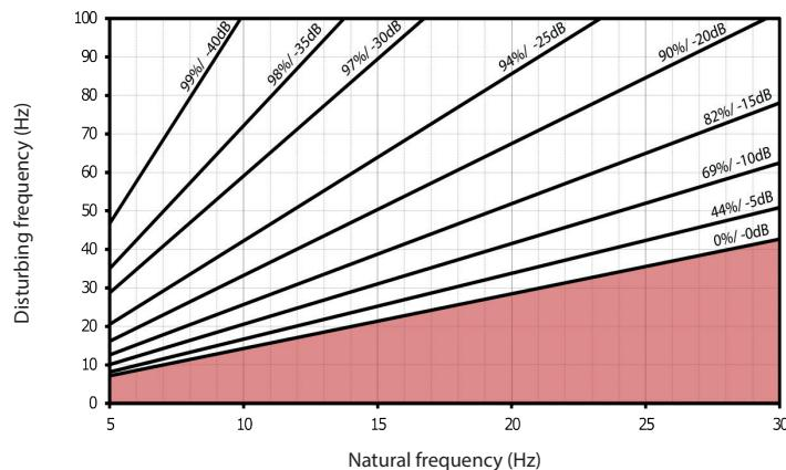
Vibration isolation efficiency by implementation of an elastic bearing made of VibraFlex® VF65 on a rigid base.
