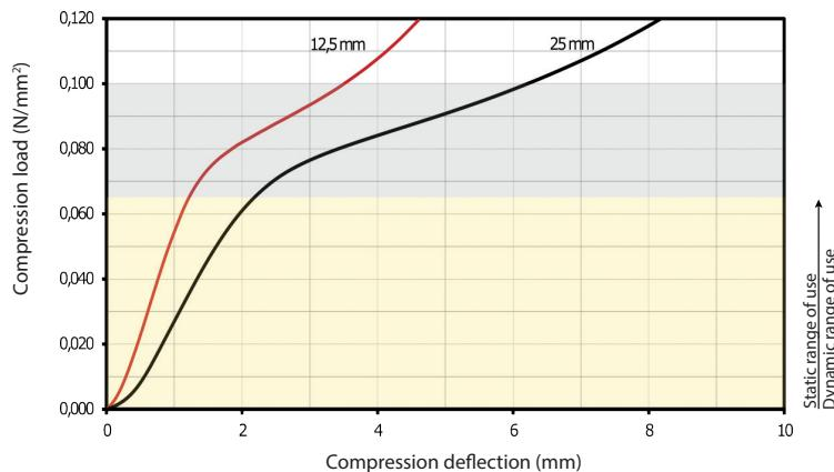
Static compression load deflection of 3<sup>rd</sup> load occurrence. Testing between flat and plane-parallel steel plates.
