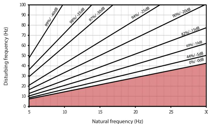
Vibration isolation efficiency by implementation of an elastic bearing made of VibraFlex® VM220 on a rigid base.
