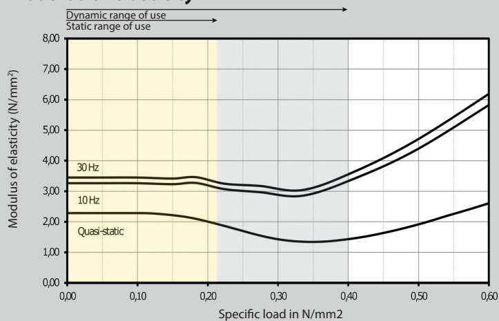
Dynamic modulus of elasticity for a sinusoidal excitation at a constant mean load and an amplitude of  $\pm 0,25$  mm.
