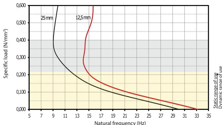
Natural frequency of a single degree-of-freedom system (SDOF System) consisting of a mass and an elastic bearing made of VibraFlex® VM220 on a rigid base.
