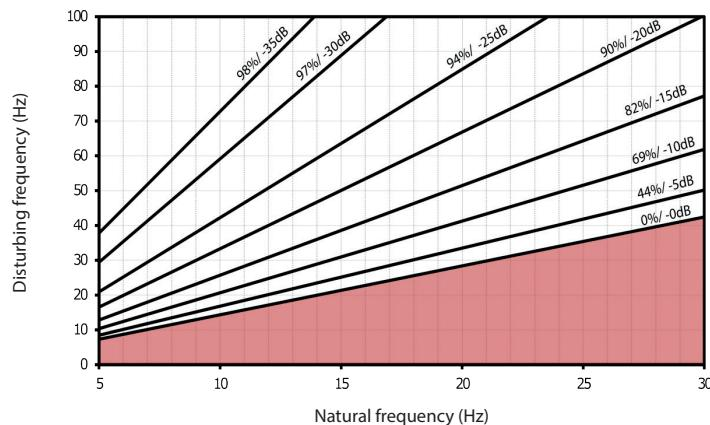
Vibration isolation efficiency by implementation of an elastic bearing made of VibraFlex® VM1200 on a rigid base.
