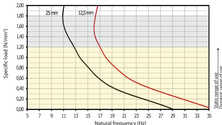
Natural frequency of a single degree-of-freedom system (SDOF System) consisting of a mass and an elastic bearing made of VibraFlex® VM1200 on a rigid base.
