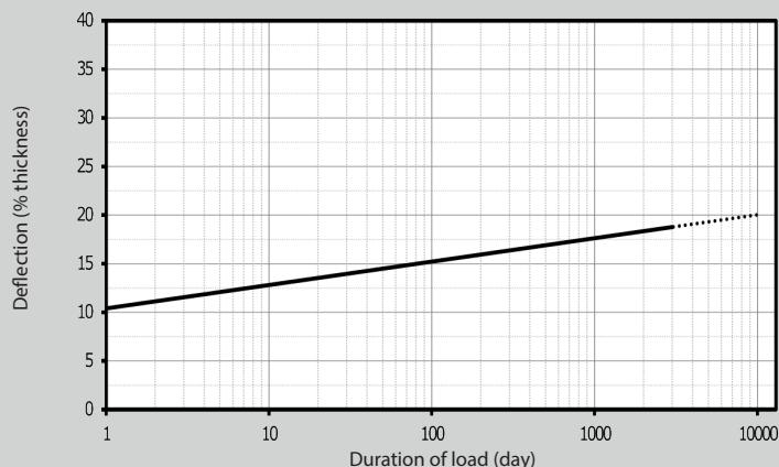
Long term creep effects occurring under long time load under room temperature.
