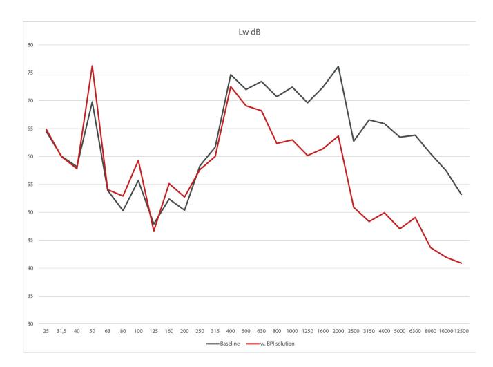
We have a long track record of successful noise reducing solutions, where we have achieved a general noise reduction of 5-12 dB(A). In the diagram below, we illustrate how a noise issue can look with and without a noise reducing solution from BPI:
